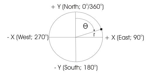
**Important Note:** In <u>surveying applications</u>, the angle (or azimuthal direction),  $\Theta$ , is measured clockwise from North.
