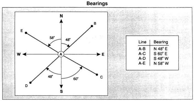
A bearing of a line or course is the angle swung from the north or south meridian in one of the four quadrants.
