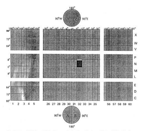
The System of UTM and UPS grid zone designations. Each quadrilateral is identified by its column number and row letter (I and O are omitted). The tinted zone is 32N. The UPS grid zones in the polar areas are sectors on each sde of the 0°-180° meridians.
