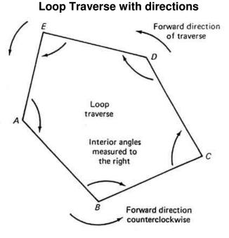
Loop traverses are best surveyed in a counterclockwise direction, with interior angles "turned" to the right.
