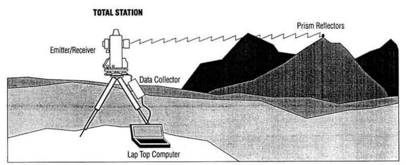
A total Station system, showing the emitter/receiver, the reflective prisms and the digital data recorder operating in conjunction with the laptop computer.
