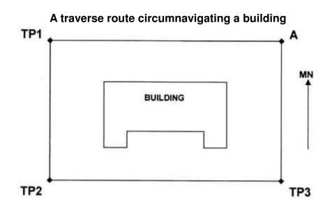
**Field Measurements:** For a Pace and Compass traverse, the actual field measurements are very straightforward. They include the Station (STN), the Magnetic North Azimuthal Direction (AZIM), the distance in paces (DIST), and any notes about the benchmark and turning points (NOTES).
