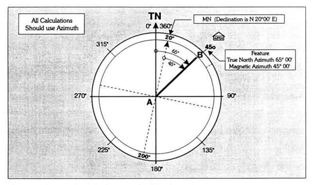
The true north azimuth and the feature are fixed, but the angle to the feature from the magnetic meridian is different.
