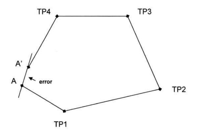
**Corrections:** Of course, plotting rarely goes well. There are just too many inaccuracies inherent in the process. However, if the last symbol does not match up with the benchmark, it can be corrected using the *proportion to station* method. This method is applied directly on the plot:
